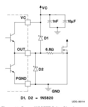
Figure 12. Power MOSFET Drive Circuit
